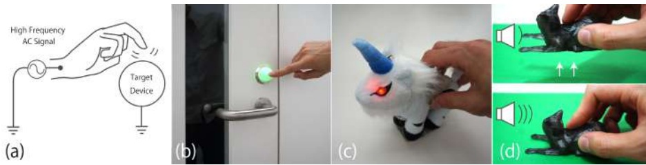
Figure 7.1: Intentiō and its applications: (a) Intentiō enables users to distribute power to electronic devices from power passing through their body. (b) Electronic and IoT devices are activated and powered by power distributed from the user. (c) Electronic stuffed toy activated by the user. The LED eyes emit light when the user touches the toy. (d) The user can adjust the amount of power distributed to the target device. Here, the volume of an electric music box is being adjusted.
