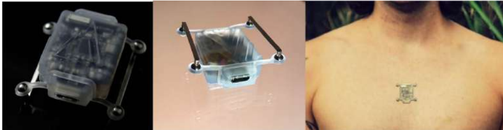
Figure 8.2: The North Sense Product [37]. The sensor vibrates when the user faces the north, and indicates the direction he/she is facing. The main device is attached to the body over the skin to the implanted attachments.
