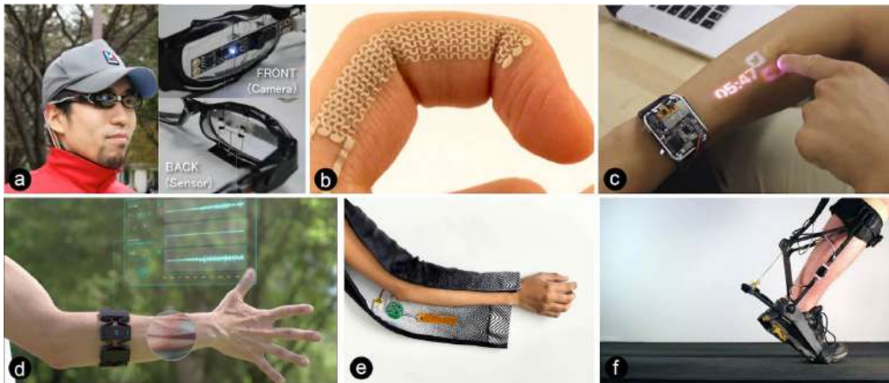
Figure 1.2: Example of Wearables. (a) Computer on an eyeglass [111]. (b) An interactive tattoo [336]. (c) A smartwatch with a projector [348]. (d) An armband for electromyographic (EMG) sensing and interaction [309]. (e) An interactive clothing [244]. (f) An exoskeleton for walking assistance [361].
