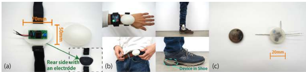
Figure 7.3: Intentiō system: (a) The design and size of the wearable device. (b) The wearable device is worn on the wrist, belt, ankle, or inside a shoe. (c) An example design of the receiving circuit. The size is not fixed, and can be designed to be the same shape as a coin cell.
